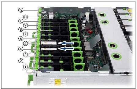
Figure 27: PCI slots with and without hot-plug functionality
